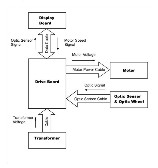
**Definition:** The main IC (also called the CPU) on the display board did not receive the optic sensor signal.
