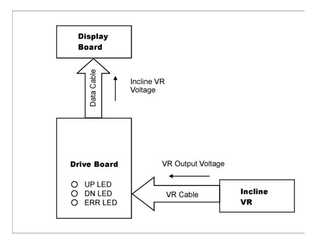
**Definition:** The display board main IC didn't receive the incline variable resistor (VR) value, or the value exceeds the set range.
