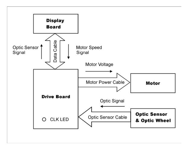
**Definition:** Speed signal error -- the speed signal from the optic sensor and the display speed setting differ.
