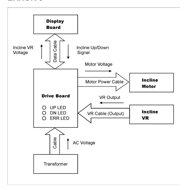
**Definition:** The incline system isn't responding to commands from the display.
