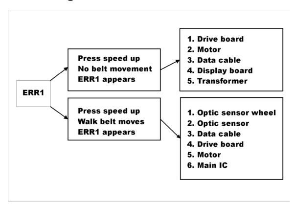
**ERR1 Condition 1**: Press speed key; walk belt doesn't move; ERR1 appears.
