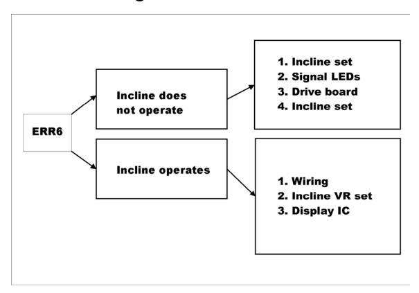
**ERR6 Condition 1:** Press incline UP or DN key; incline doesn't operate; ERR6 appears.
